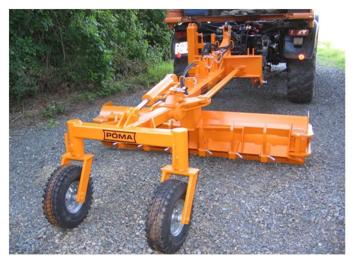
With the PÖMA-Grader H225 ESP we complete our, over many years proven road-buildingmachines, with a cheap, professional deployable unit. New in this series is the sideways parallel motion of the device using a guide-bar. Thereby the subsequent support wheels always stay behind the Grader-shield.
